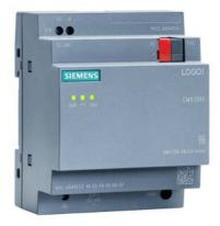
LOGO! CMK2000 Communication module for integrating the LOGO! 8 "in the building system bus KNX;" connection 24 V DC 0.04A 1 RJ45 port for Ethernet 50 communication objects time-of-day synchronization Configuration/diagnostics via web interface
