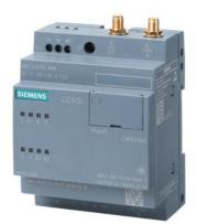
LOGO! CMR2040 communication module for connection LOGO! 8 to LTE network; 1 RJ45 port for Ind. Ethernet connection to LOGO! 8; 2xDI; 2xDQ; Write/read access to LOGO! tags; Text message sending/ receipt; E-mail sending; Position detection GPS; Time synchronization/ forwarding with real-time clock; Configuration/diagnostics via web interface; Remote access via OpenVPN/HTTPs, DynDNS, observe national approval! Manual available as a download
