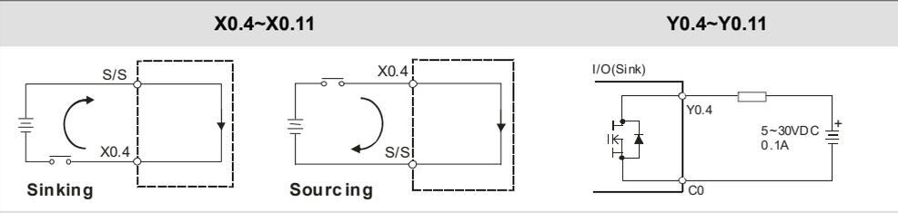
X0.0+~X0.3+/X0.0~-X0.3-: 5VDC, differential Y0.0+~Y0.3+/Y0.0~-Y0.3- : 5VDC, 20mA, differential
