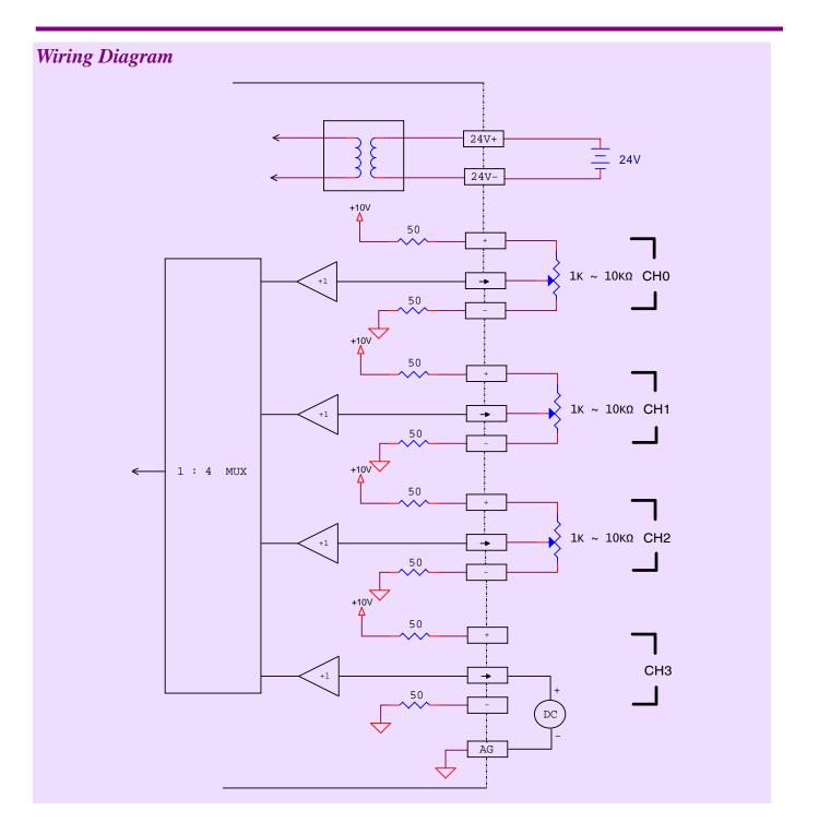
In the above sample wiring, the wiring of CH0~CH2 are for potential meter, while the CH3 is for  $0 \sim 10V$  single ended voltage type signal. The internal serial resistors at upper or lower leg for each channel are for wire broke detection purpose. The too big or too low input value indicates the wire broke situation.
