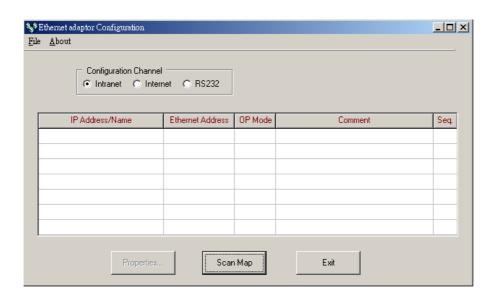
Click the 'Scan Map' button then start the scanning of Ethernet module. All the modules detected will be shown in the table. The remaining procedures will be left until section 5.3.4.
