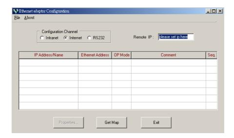
At this time can input the remote IP address of the Ethernet module desired for configuration. After click the 'Get Map' button, it will start to connect Ethernet module. When the connection is established will show the information regard the connected Ethernet module in the table at the middle of window.
