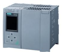
\*\*\* spare part \*\*\* SIMATIC S7-1500F, CPU 1518F-4 PN/DP ODK, central processing unit with ODK runtime interface, 9 MB work memory for program and 60 MB for data, 1st interface: PROFINET IRT with 2-port switch, 2nd interface: PROFINET RT, 3rd interface: PROFINET basic services, 4th interface: PROFIBUS, 1 ns bit performance, SIMATIC Memory Card required
